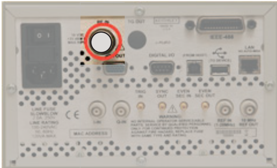
Figure 3 V2820A-SPI with 50 \Omega termination
